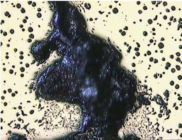
Fig. 5. Defects in cast iron: loss of nodularity around a cavity (on the left) and dendrites grown on the wall of a shrinkage cavity (on the right)
