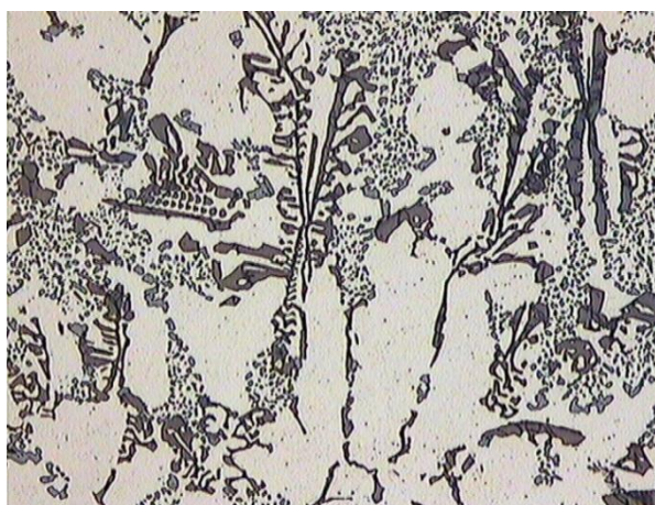
Fig. 3. Light microscopy and SEM images of intermetallic phases in gravity cast Aluminium-Silicon alloys
