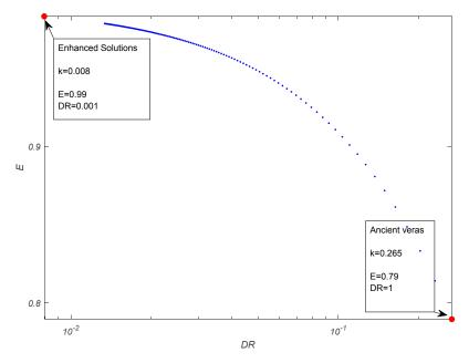
**Figure 3.** Cistern efficiency (E) according to probability analysis (Equation (8)). Typical ancient vera draining water from campiello only vs. enhanced solutions (red dots) and intermediate solutions (blue dots) obtained for different values of b and plotted versus demand ratio (DR).
