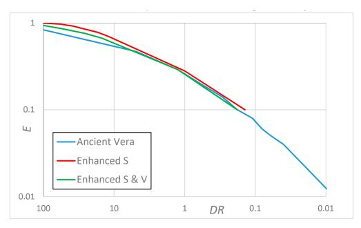
Figure 4. Cistern efficiency vs. demand ratio. Results of numerical simulation.
