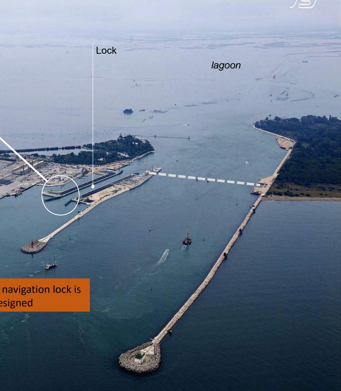
A new gate of the navigation lock is being designed
