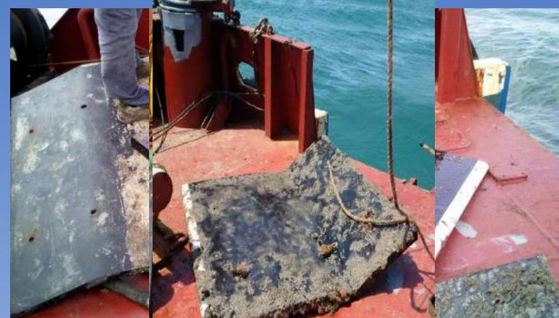
During the test performed in may 2016, the reinforced rubbers have been deformed due to the presence of sediments between the caissons and the gates
