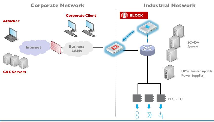
The integration between SCADAguardian and the perimeter firewall provides additional protection against these types of attack
