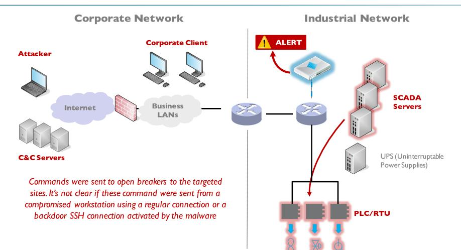
NOZOMI SCADAguardian monitors process commands and variables, alerting on critical or undesired conditions
