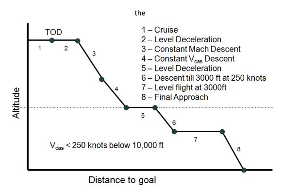
Fig. 10 Descent profile for a commercial aircraft
