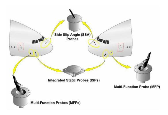
Fig.4 Example of Probes location in an A380
