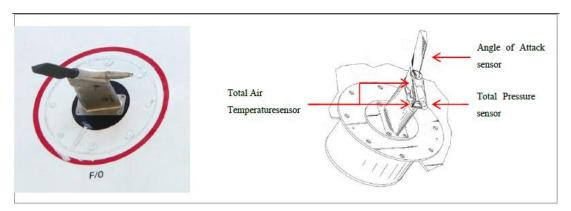
Fig.5 Example of A380 Multi-Function Probes
